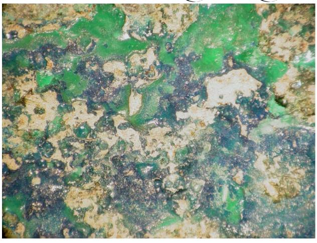
This is a micrograph taken from the external surface of the vessel. There is both malachite and azurite crystal growth. Small pieces of the patina were removed from randomly chosen areas. The crystals appeared to grow directly out of the metal as expected on a natural patina. Flame tests of the removed patina were positive for the presence of copper.
